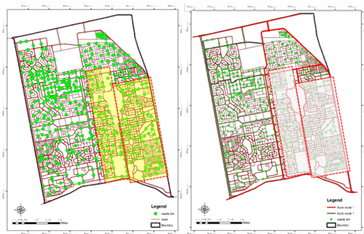
Fig no.3 (Left), Proposed locations of waste bins, Fig no.4 (Right), Route optimization with proposed waste bins Source: By the authors using GIS.
